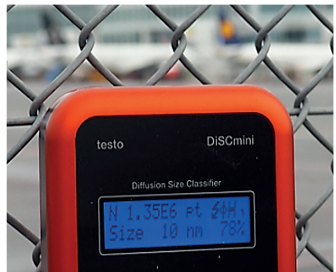
Figure 6 Discmini measurement close to the apron of the Munich Airport shows a UFP concentration ( \leq 10 \text{ nm} ) of 1.35 Mio. \text{p}/\text{cm}^3 . Source: BV Freising
